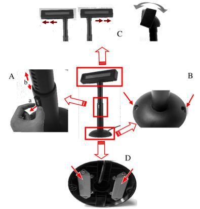
Picture A is going to describe how to adjust the height of customer displays:
